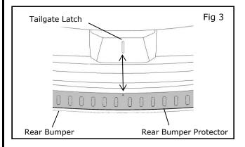
4) Dry fit bumper protector on vehicle by aligning bumper protector centering arrow with tailgate latch.
